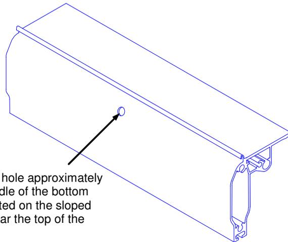
Drill 3/16" hole approximately in the middle of the bottom rail. Located on the sloped portion near the top of the extrusion.
