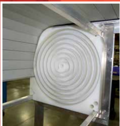
Cover stores neatly inside the bed using this simple coil system
